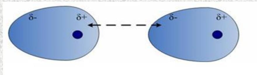
Attraction forces exist between the two induced dipole atoms
