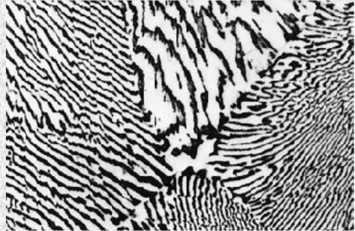
microstructure of a lead–tin alloy of eutectic composition
