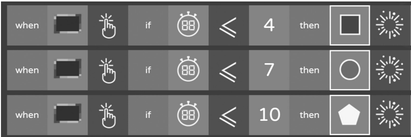
11.10 Rules that involve a timer. The first specifies that a click causes a blue square to be created only if no more than four seconds elapsed since the beginning of the execution.
