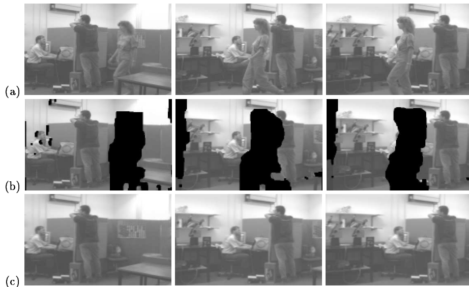
Fig. 3. Dominant motion selection and outlier rejection. (a) 3 representative frames from the sequence. There are two motions present – that induced by the panning camera, and that induced by the walking woman. (b) Outlier pixels detected in those frame are marked in blacks. Those pixels found to be moving inconsistently with the detected dominant motion. Those pixels correspond to the walking woman, to her reflection in the desk, to the boundaries of the image frames, and to some noisy pixels. (c) Full reconstructions of the dominant layer (the background) in all frames. The girl, her reflection, and the noise are removed from the video sequence by filling in the black regions with gray-level information from other frames according to the computed dominant background motion.
