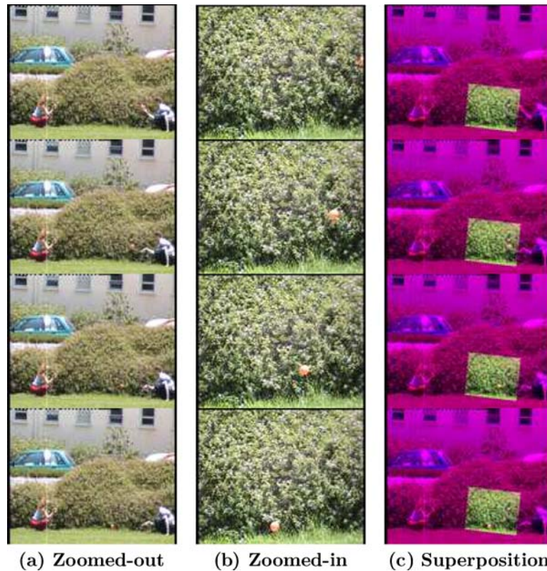
Figure 4. Alignment of sequences obtained at different zooms. Columns (a) and (b) display four representative frames from the reference sequence and second sequence, showing a ball thrown from side to side. The sequence in column (a) was captured by a wide field-of-view camera, while the sequence in column (b) was captured by a narrow field-of-view camera. The cameras were located next to each other (the spatial transformation was modeled by a homography) and the ratio in zooms was approximately 1:3. The two sequences capture features at significantly different spatial resolutions, which makes the problem of inter-camera image-to-image alignment very difficult. The dynamic information (the trajectory of the ball’s center of gravity), on the other hand, forms a powerful cue for alignment both in time and in space. Column (c) displays superposition of corresponding frames after spatio-temporal alignment, using the algorithm of Section 3 for estimating the homography and the temporal correspondence between the two sequences. The dark (pink) boundaries in (c) correspond to scene regions observed only by the reference (zoomed-out) camera.
