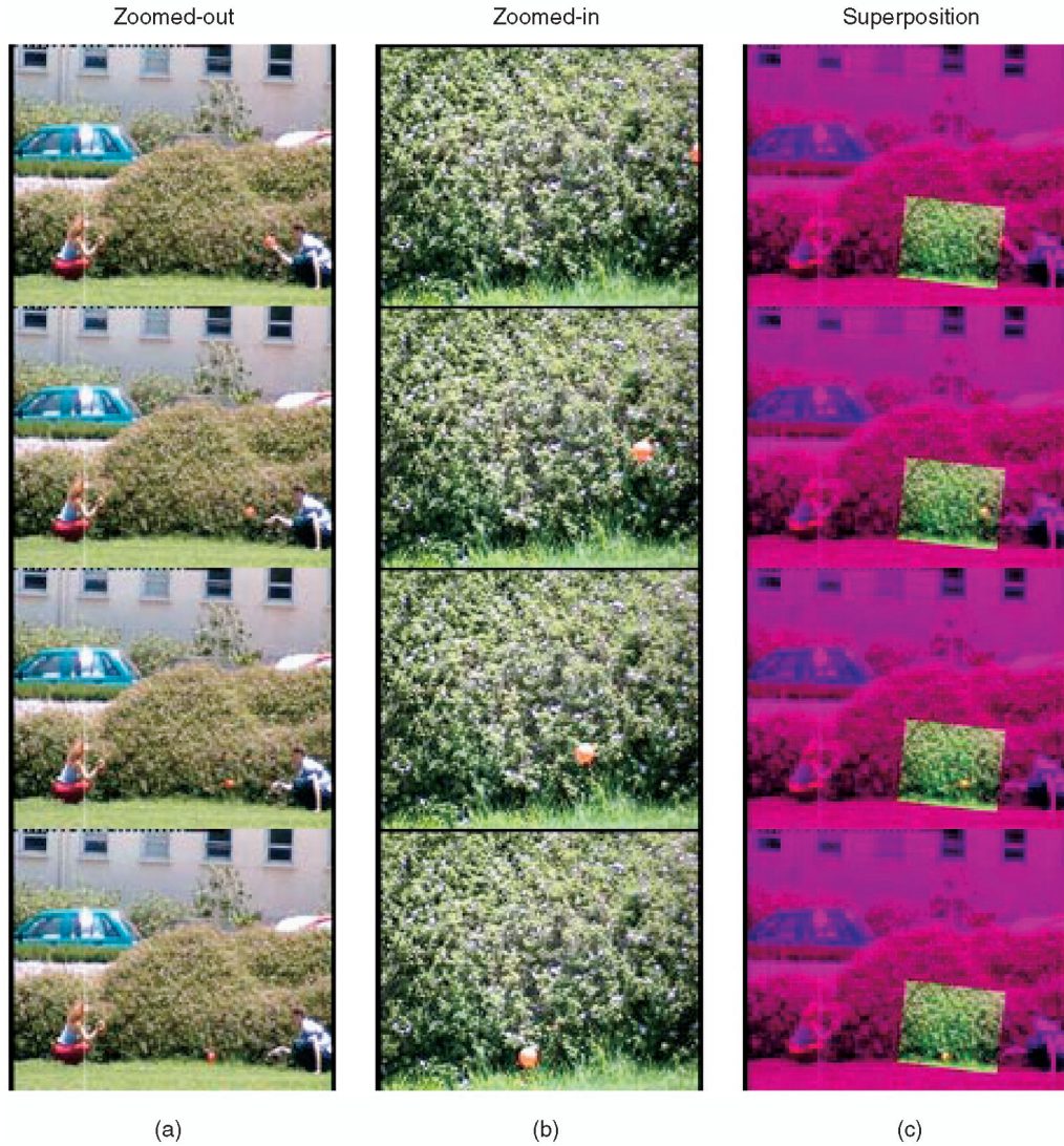
Fig. 12. Super-position. Alignment of sequences obtained at different zooms. Columns (a) and (b) display four representative frames from the reference sequence and second sequence, showing a ball thrown from side to side. The sequence in column (a) was captured by a wide field-of-view camera, while the sequence in column (b) was captured by a narrow field-of-view camera (the ratio in zooms was approximately 1 : 3). The two sequences capture features at significantly different spatial resolution, which makes the problem of intercamera image-to-image alignment very difficult. The dynamic information (the ball trajectory) on the other hand, forms a powerful cue for alignment both in time and in space. Column (c) displays superposition of corresponding frames after spatio-temporal alignment, using the feature-based algorithm of Section 3.1. The dark pink boundaries in (c) correspond to scene regions observed only by the reference (zoomed-out) camera. For full color sequences, see www.wisdom.weizmann.ac.il/Seq2Seq .
