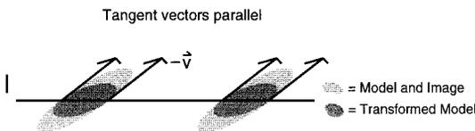
Figure 4. Two model regions lead to non-unique affine transformations when a line  $l$ , exists such that the tangents at all intersection points are parallel. In this case, the regions can contract towards  $l$  in the direction  $\vec{v}$ .
