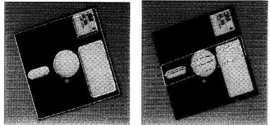
Figure 13. Matching the diskette model to a novel image of the diskette using two degenerate regions only (the left and the lower right, left figure: similarity,  $\lambda = -1.15$ , right: affine,  $\lambda = -0.55$ ).
