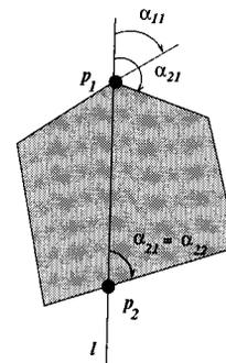
Figure 8. Notation: when  $l$  intersects the boundary of a polygon at a vertex (as in  $\vec{p}_1$ )  $\alpha_{11}$  and  $\alpha_{21}$  are the angles between the two sides emanating from  $\vec{p}_1$  and the positive direction of  $l$ . When  $l$  intersects the boundary of a polygon at a side (as in  $\vec{p}_2$ )  $\alpha_{21} = \alpha_{22}$  is the angle between the side and the positive direction of  $l$ .
