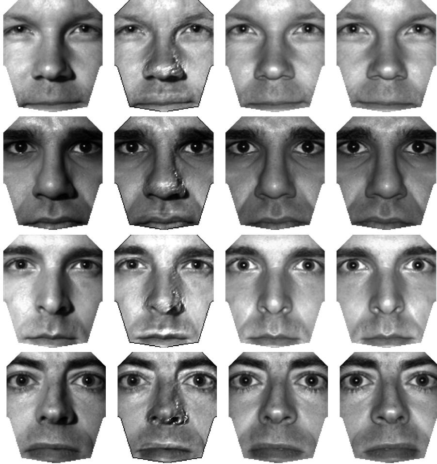
Fig. 5. The four different rows correspond to four different faces from the Yale face database B. The first column contains renderings of faces with side illumination Az = 20^\circ and El = 10^\circ . The second column contains images rendered from images in column 1 using the depth recovered by our algorithm. The faces in the second column should be similar to the frontally illuminated faces in column 3 (one should ignore shadows present in the rendered images, because such a simple cancellation scheme is not supposed to cancel them out). Finally, the last column contains frontally illuminated faces from column 3, flipped around their vertical axis. By comparing two last columns, we can see noticeable facial asymmetry, even in the case of the three best faces. For the fourth face asymmetry is rather significant, specially depth asymmetry near the nose, causing rather big errors in the reconstructed depth, as can be seen in Fig. 4.
