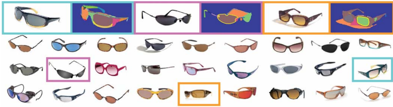
Figure 4 | Similarity search by parts. Top: three example queries (cyan, pink, orange frames) with the original images on the left. The segmentation of each image is shown on the right in each frame, with the target query segment (user-selected) outlined in yellow: lower flank of left frame, right
