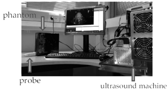
Fig. 9. Lab setup: ultrasound system, probe and cardiac phantom.
