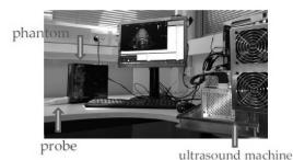
Fig. 4: Lab setup: Ultrasound system, probe and cardiac phantom.
