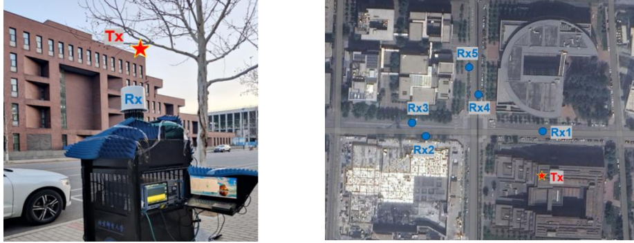
(a) Scenario of XL-MIMO channel measurement (b) Layout of XL-MIMO channel measurement Fig. 4.3 XL-MIMO channel measurement [184].
