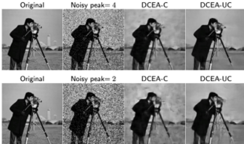
Fig. 6. Illustration of an image corrupted by different levels of Poisson noise and the resulting denoised images produced by the unfolded DCEA-C and DCEA-UC. Figure reproduced from [51] with authors' permission.
