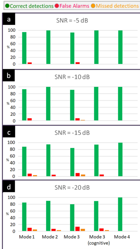
Fig. 18. Statistical performance of different array configurations in a CoSUMMeR prototype over 100 realizations of randomly spaced target scenes.
