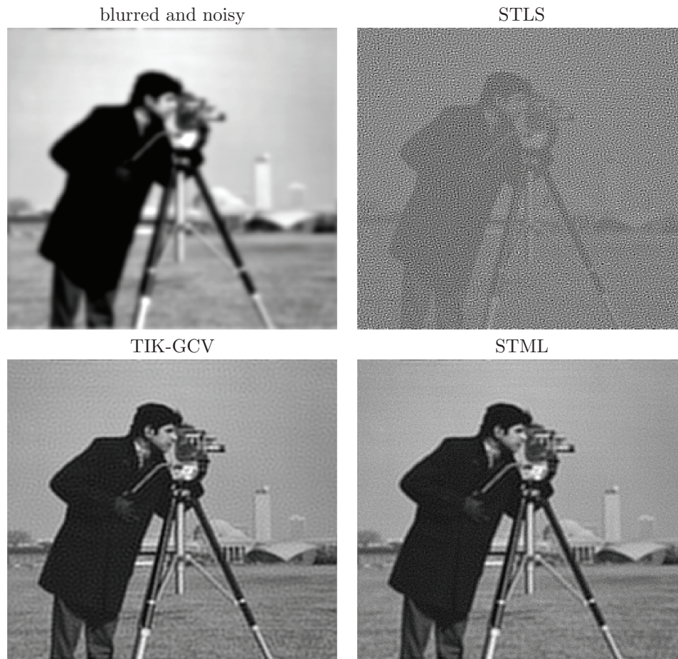
FIG. 5.1. Deblurring of the cameraman. Top left: blurred and noisy image. Top right: naïve reconstruction which coincides with the STLS estimate. Bottom left: Tikhonov with GCV parameter choice. Bottom right: the STML solution.
