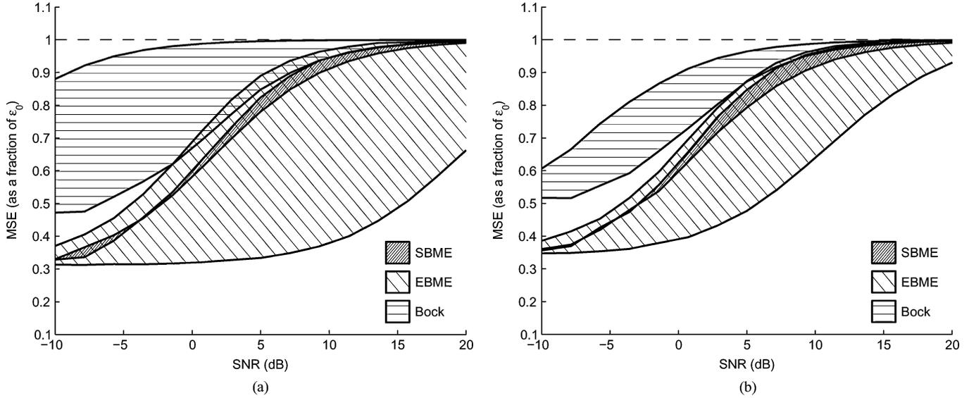
Fig. 6. Range of possible MSE values obtained for different values of  $\mathbf{x}$ , as a function of SNR.  $\mathbf{H} = \mathbf{I}$  for both parts. (a)  $m = n = 15$ , with eigenvalues of  $\mathbf{C}_w$  distributed uniformly between 1 and 0.01, resulting in an effective dimension of 7.6. (b)  $m = n = 10$ , with  $\mathbf{C}_w$  containing five eigenvalues of 1 and five eigenvalues of 0.1, resulting in an effective dimension of 5.5.
