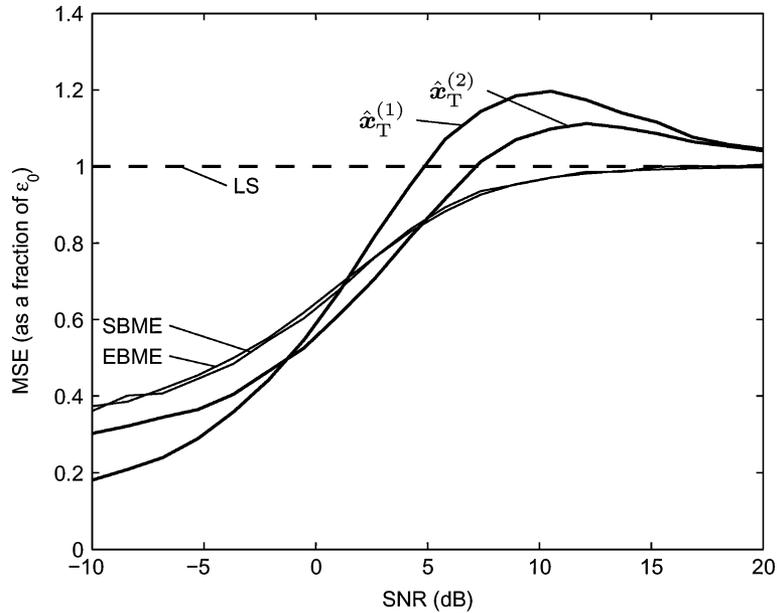
Fig. 4. Comparison between Tikhonov regularization, LS, and BME. The Tikhonov estimators  $\hat{\mathbf{x}}_T$  are seen to perform worse than the LS estimator at high SNR, whereas the BMEs dominate the LS method.
