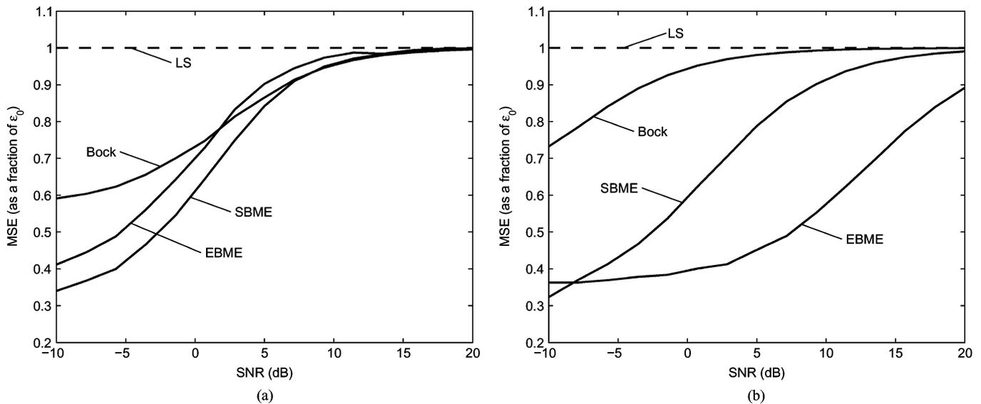
Fig. 5. MSE versus SNR for a typical operating condition: effective dimension 5.8,  $m = n = 15$ . (a) Parameter vector  $\mathbf{x}$  in direction of maximum noise. (b) Parameter vector  $\mathbf{x}$  in direction of minimum noise.
