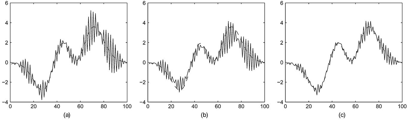
Fig. 2. Estimation of a signal from measurements of its DCT. In this example, high-frequency components have a much higher noise variance than low-frequency components. Dashed line indicates original signal; solid line indicates estimate. (a) LS estimate; (b) spherical BME, resulting in a shrinkage factor of 0.79; (c) ellipsoidal BME, with shrinkage in the range 0.44–0.98.
