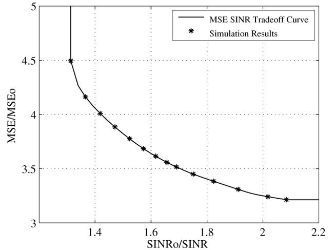
Fig. 6. MSE-SINR tradeoff for INR = 20 dB, SNR = 0 dB and  $b = 0.7$ . The diagonally loaded sample covariance matrix  $\hat{\mathbf{R}}_{\text{dl}}$  is used in lieu of the true covariance matrix  $\mathbf{R}_{i+n}$ .
