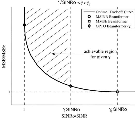
Fig. 1. Qualitative example of the optimal tradeoff curve in the MSE-SINR plane.
