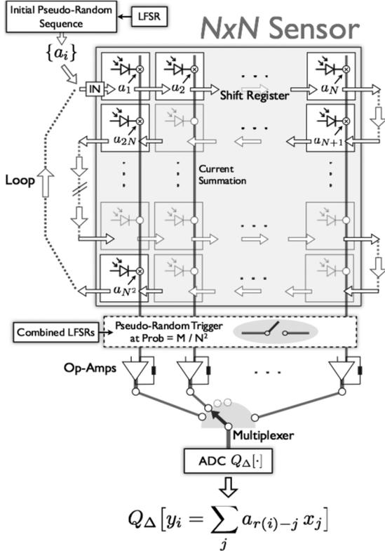
Fig. 5. Schematic for the microelectronic architecture of the convolution-based compressive imager. The acquisition device effectively implements a subsampled circulant CS matrix. Here,  $Q_\Delta$  denotes the quantization operation with resolution  $\Delta$  (taken from [95]).
