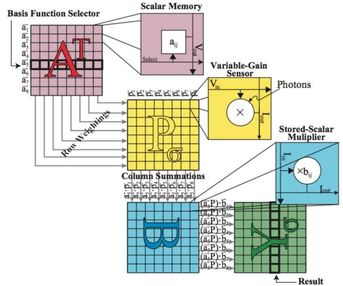
Fig. 6. Schematic for the compressive analog CMOS imager. The acquisition device effectively implements a separable CS matrix (taken from [99]).
