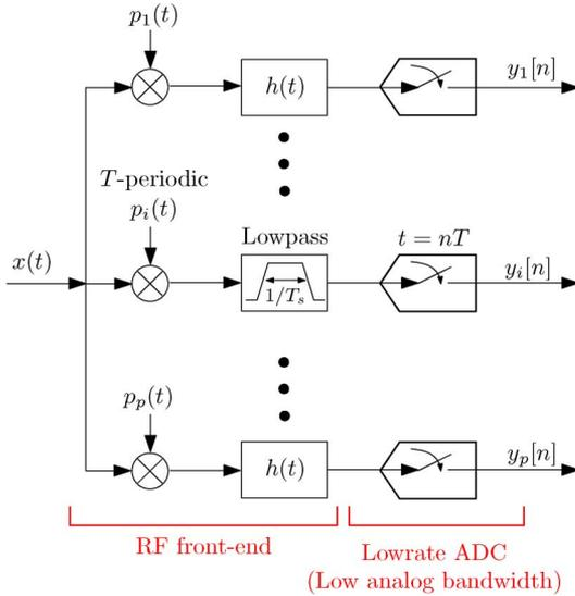
Fig. 13. Block diagram of the modulated wideband converter. The input passes through  $p$  parallel branches, where it is mixed with a set of periodic functions  $p_i(t)$ , lowpass filtered and sampled at a low rate (taken from [9]).
