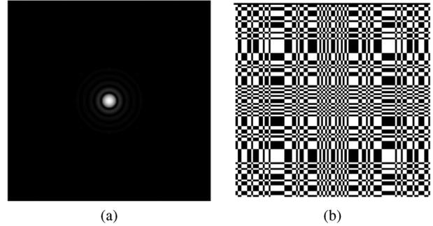
Fig. 4. Compressive imaging via coded aperture. (a) Example of an ideal point spread function for a camera with a pinhole aperture. The size of the support of the function is dependent on the amount of blur caused by the imager. (b) Coded aperture used for compressive imaging (taken from [94]).
