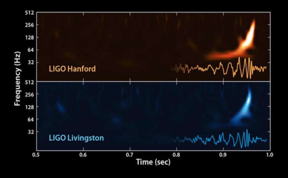
The time-frequency distribution of the gravity waves from the two LIGO interferometers
