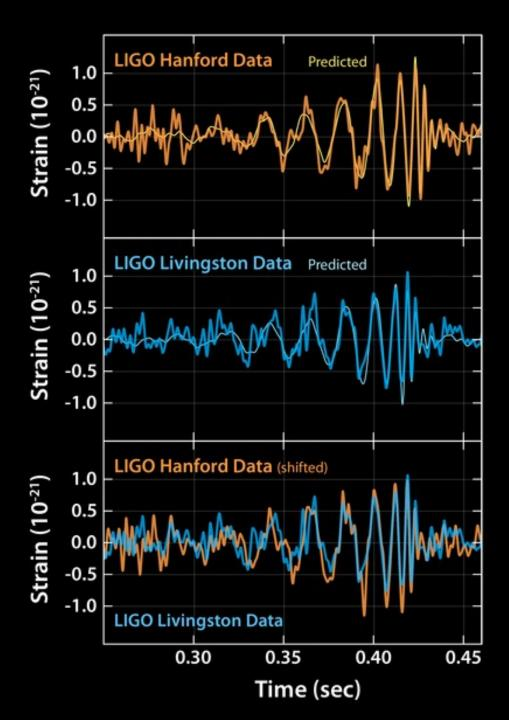
The data is filtered to obtain only the frequency of the black-holes rotation, Then the time delay is best fitted.
