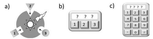
Schematic representation of (a) a 3-input molecular keypad lock (chemical inputs are denoted as 1, 2, and 3), (b) a 3-input electronic keypad lock, and (c) a conventional electronic keypad lock. Credit: Rout, et al. ©2013 American Chemical Society
