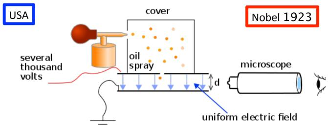
Millikan oil droplets experiment to determine electron charge Above: schematics Below: photo of the instrument
